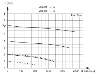
Ports with interchangeable 1/4 threaded cartridges
